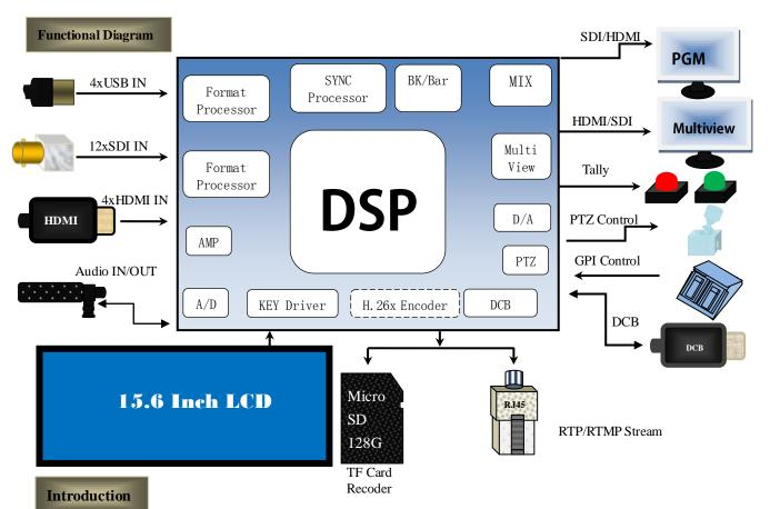
A dedicated switcher for broadcast, TV and studios, it is the first choice for large-scale live broadcasts. The twenty-channel switcher integrates multiple control methods. Special effects and transition methods can be set through the keyboard. The built-in menu display function can set up the equipment more intuitively and efficiently. The joystick can control the distance and distance of the camera.
