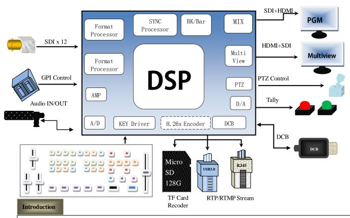
The HDS6312, a dedicated switcher for Broadcast & TV / studio, adopts a portable integrated design, metal shell, small size and light weight, which can be applied to the video special effect switching requirements of small scenes. The device integrates multiview processor, special effect generator, audio processor, control keyboard and other common switcher components.
