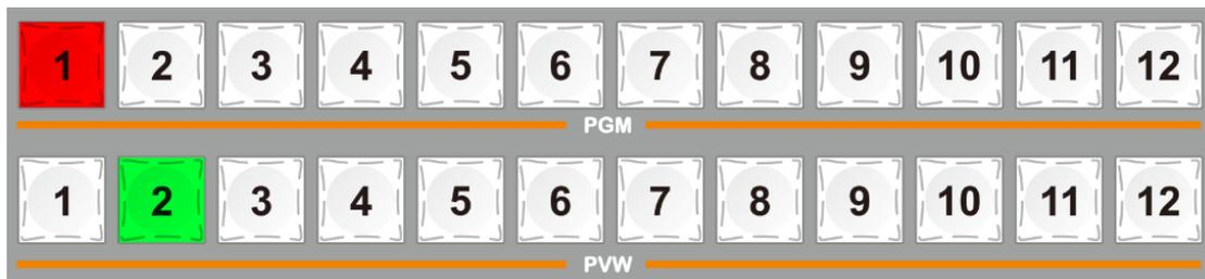
If you want to display the source of the SDI1 interface on the PVW, the source of the SDI2 interface is displayed on the PGM press the 1 button directly in the PVW area, and press PGM to press 2. As shown above
