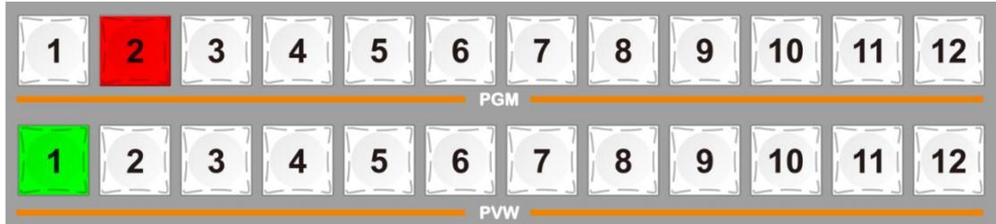
Press the selection in the PGM area as shown above, and the button will turn red (live). Pressing PVW will display green (pre-supervised).
