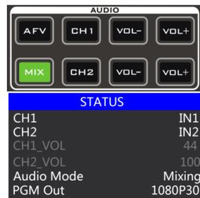
2. The mixing assigned channels are IN1、IN2、IN3、IN4、PHONE\_IN、MIC\_IN1、MIC\_IN2. Under the mixing assignment mode, there are two more audio embedding functions; PHONE\_IN means 3.5mm stereo audio interface, MIC\_IN means 3.5mm microphone audio interface; PGM live output can mix two audio channels at any time, and the volume of the two audio channels can also be adjusted separately.
