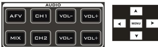
You can also press MIX (showing green light) in the key panel, then press the "up and down" buttons of the menu button to enter the audio channel selection, press the "down" button to enter the CH1 channel, click "MENU" to enter the audio source selection, audio The source can be selected from IN1、IN2、IN3、IN4、PHONE\_IN、MIC\_IN1、MIC\_IN, after confirming the selection, press "MENU" to exit; as shown in the right figure, the audio source of the first channel is from IN1-HDMI1 becomes IN4-HDMI4.
